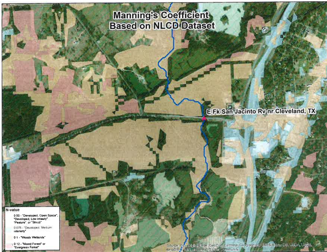
Figure 14. The graphic shows land use type which is erroneously reported in the NLCD. At this location, the NLCD raster shows 'Developed – Open Space/Low Intensity' in the majority of the area. The GIS tool initially assigns a Manning's n-value of 0.013 to this, assumed to represent paving, which is then constrained to a minimum value of 0.05. As seen in the imagery, most of the area is either dense woods, which should be written as 0.12 according to the tool, or woody wetlands with dense tree cover, which should be written as 0.1 according to the tool. Correcting these values then adjusting according to the recommendations provided in the executive summary raises the water surface elevation to within 0.5 foot of the Cleveland gage reading during Harvey.
