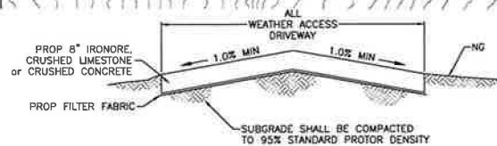
ALLWEATHER DRIVEWAY CROSS-SECTION N.T.S.
